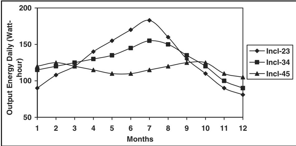
Figure 8: Daily output energy of the module in GIK Institute over the year for the selected module inclination angles of 23°, 34° and 45°. (1 is January and 12 is December)
