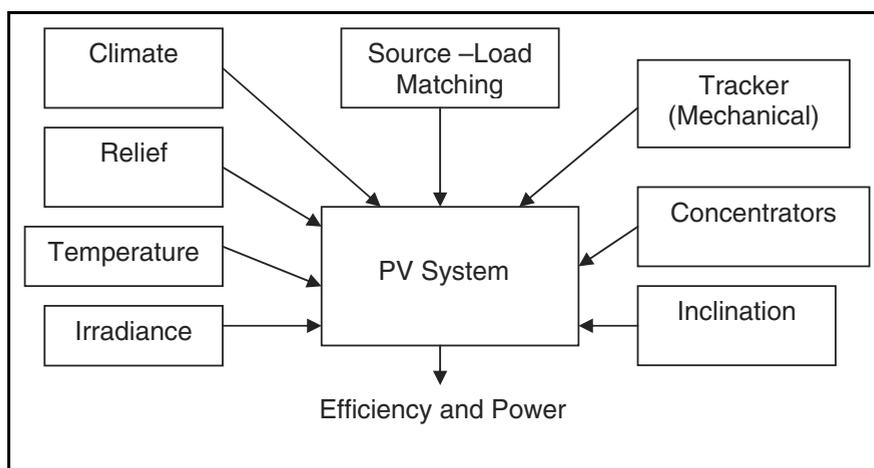
**Figure 1:** Dependence of PV system's efficiency on different factors.
