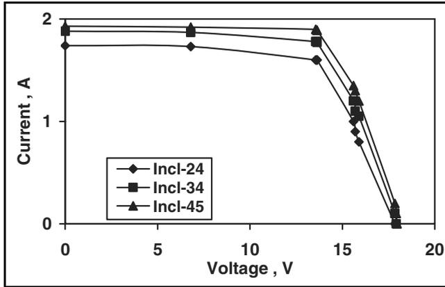
Figure 5: Current-voltage characteristics of the module measured at noon time (12:00) on a clear day for different module's inclination angles, i.e. 23°, 34° and 45°
