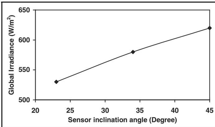
Figure 6: Global irradiance for sensor's inclination angles 23°, 34° and 45° at noon time (12:00) for a variably cloudy day
