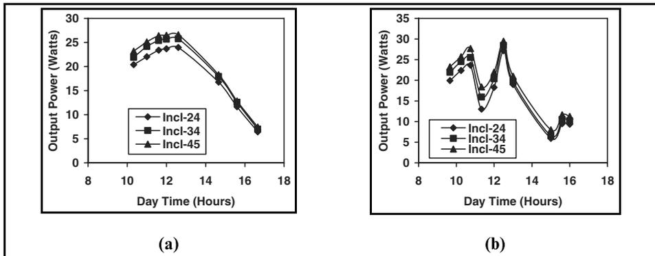
**Figure 4:** Output power vs day time relationship for the one module for different module’s inclination angles, i.e. 23°, 34° and 45°: (a) at clear day, (b) variable cloudy day
