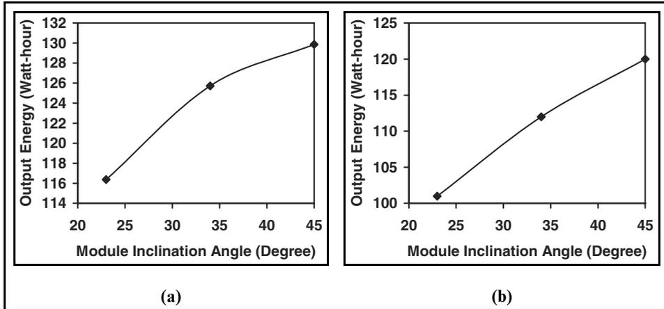
**Figure 7:** Module's output energy for module's inclination angles 23°, 34° and 45° for; (a) a clear day, (b) a variably cloudy day.
