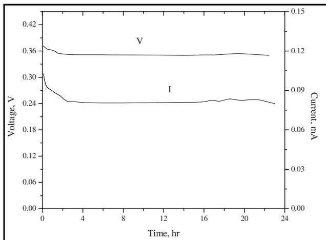
**Figure 6:** Discharge voltage/current-time behavior for 10.0 wt% concentration of orange dye in aqueous solution
