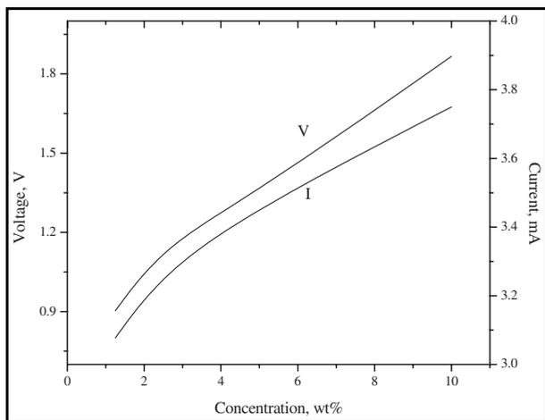
Figure 4: Open circuit voltage/short circuit current versus orange dye concentration curves for zinc/orange dye aqueous solution/carbon cells
