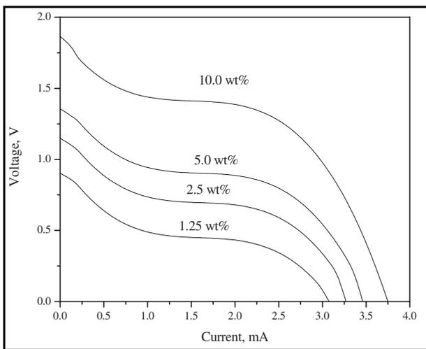
Figure 3: Voltage versus current discharge characteristic of zinc/orange dye aqueous solution/carbon cells for different concentrations
