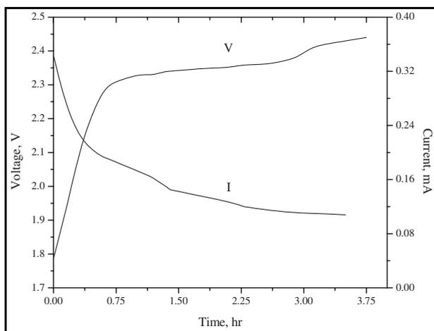
**Figure 5:** Charge voltage/current-time curves for 10.0 wt% concentration of orange dye in aqueous solution
