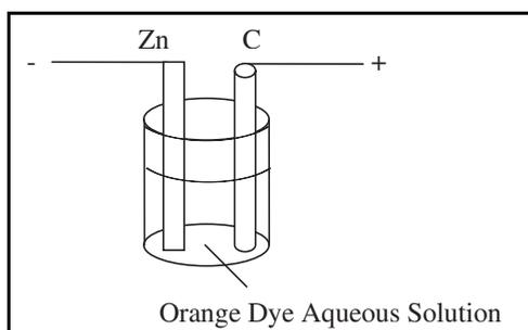
Figure 2: Schematic diagram of Zn/orange dye aqueous solution/carbon cell
