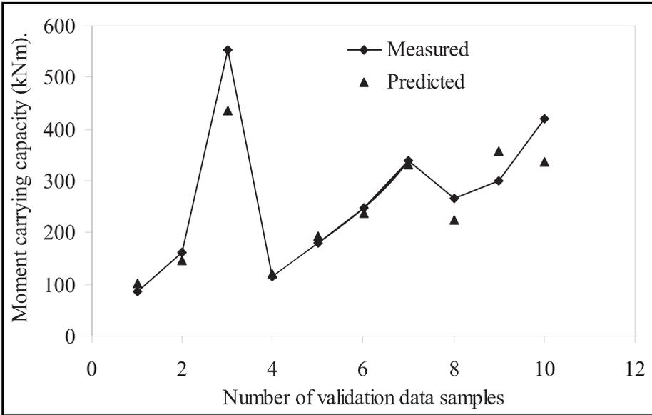
Figure 5. Comparison of the measured and predicted moment carrying capacities in the validation phase
