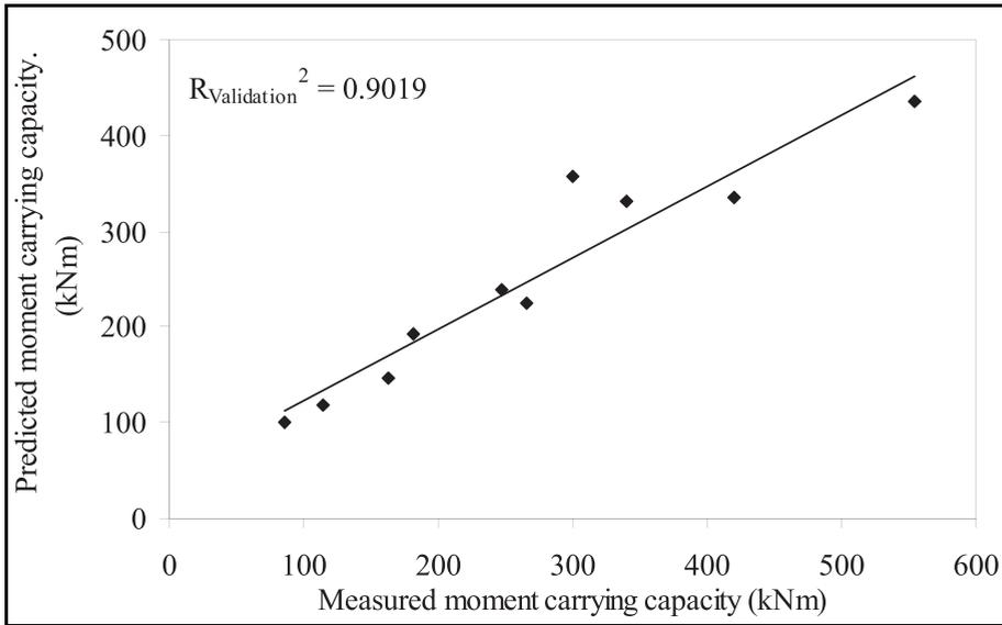
**Figure 8.** Correlation between the measured and predicted moment carrying capacities in the validation phase
