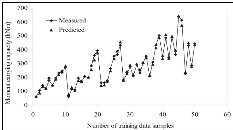
**Figure 3.** Comparison of the measured and predicted moment carrying capacities in the training phase
