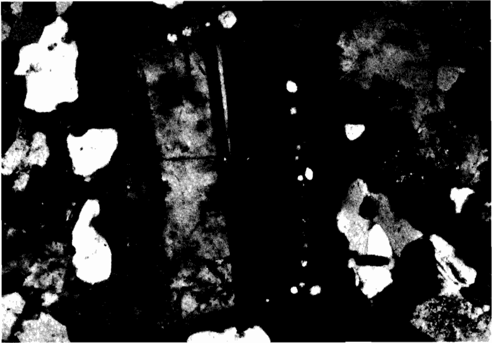
Fig. 3. Zoned plagioclase crystal showing porphyritic texture. Crossed nicols. \times 40 .
