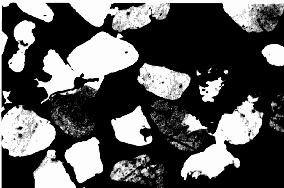
Fig. 7. Quartz grains in ferruginous clay matrix, inhibiting quartz overgrowths. Note marked marginal corrosion of several quartz grains (crossed nicols, \times 10 ). Selected sand sample from traverse y-y' (see Fig. 1).
