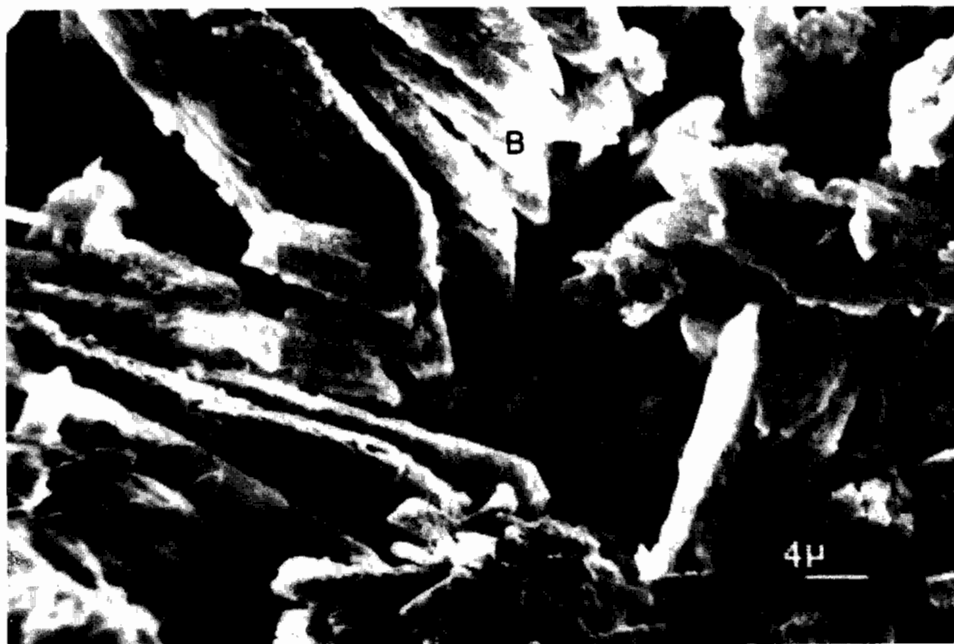
Fig. 2. SE micrograph of bundles of needle-like bassanite crystals (B) showing hexagonal morphology. Surface sample collected at the beginning of the dry season after the rains, Al-Khiran pans.
