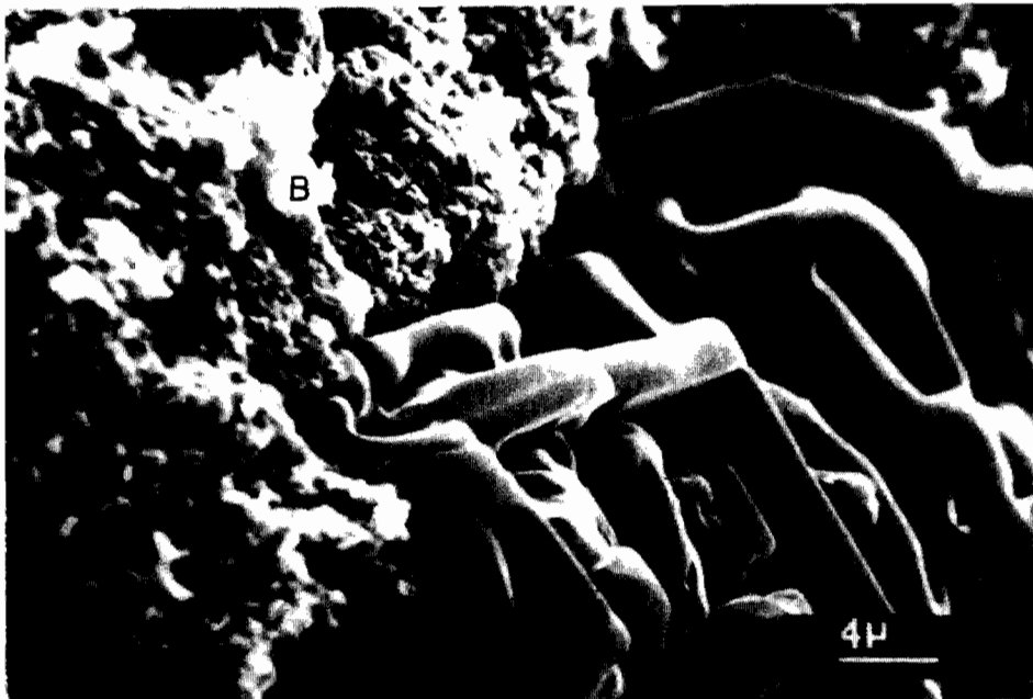
Fig. 9. SE micrograph of a broken surface of a partially altered gypsum grain. Note cryptocrystalline bassanite (B) on the left and the still unaltered core of the gypsum crystal, an evidence that the transformation proceeds centripetally from the outside to the inside of the crystal. Al-Khiran.
