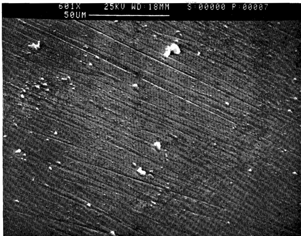
Plate 3. Scanning electron micrograph (601 X) showing the morphological features of corrosion formed on the surface of carbon steel after exposure for 50 h in export grade Kuwaiti crude oil containing 10 ppm 2-amino-thiazole (ATH).
