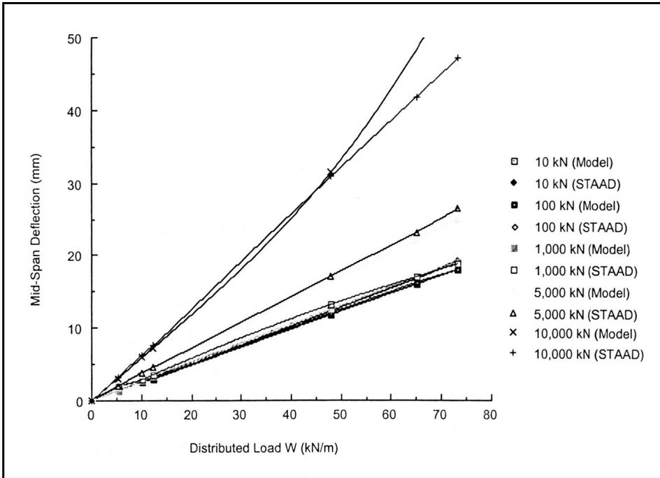
**Figure 9.** The mid-span deflections of the beam-column example under combined distributed and concentrated axial loads using the proposed model and STAAD (9 cycles).
