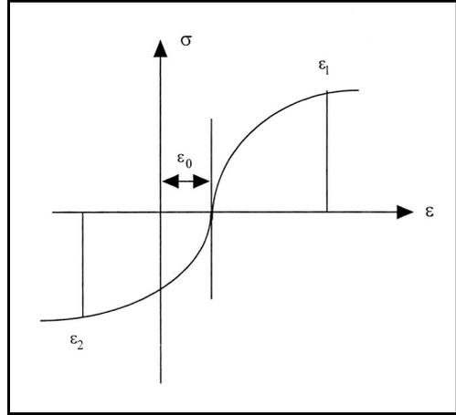
Figure 2. The shifted inelastic stress-strain diagram
