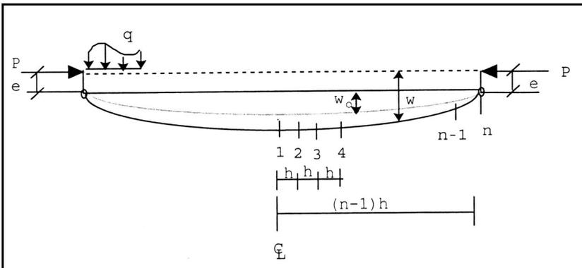
Figure 7. Finite Difference discretization of a symmetric simply-supported beam
