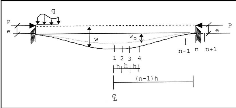
**Figure 10.** The Finite Difference discretization of a symmetric fixed beam
