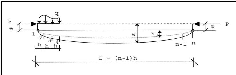
Figure 1: Finite difference modeling of a simply supported beam.
