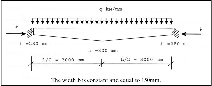
**Figure 8.** Simple beam used to verify the proposed model
