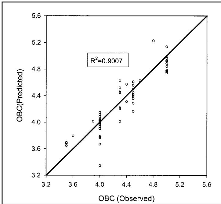
Fig. 9. The Correlation of Predicted to Observed OBC for Asphalt-Concrete Type I, II, III, and IV.
