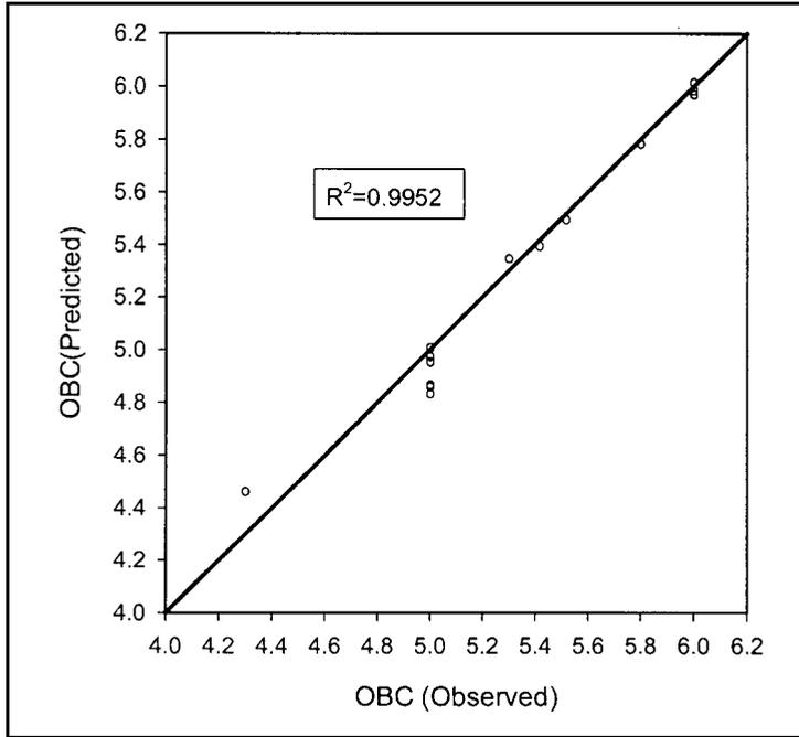
Fig. 8. The Correlation of Predicted to Observed OBC for Asphalt-Concrete Type PMS.
