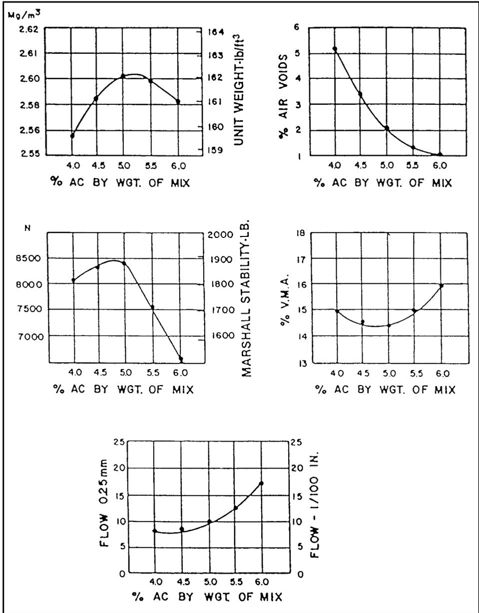
Fig. 1. Typical Marshall Test Results (AI 1988).
