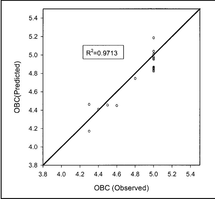
Fig. 6. The Correlation of Predicted to Observed OBC for Asphalt-Concrete Type III.
