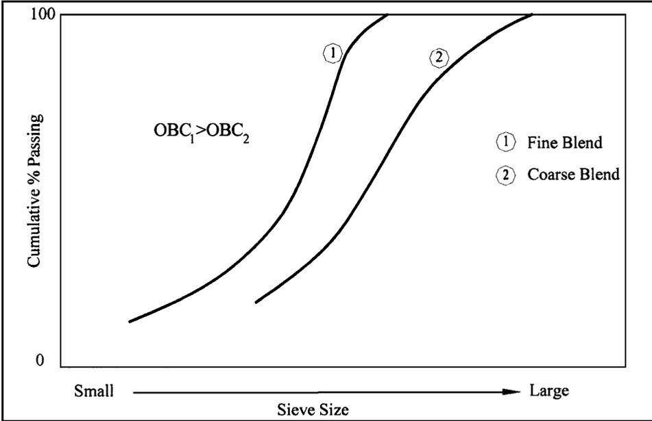
Fig. 3. Size Gradation of Two Aggregate Blends.
