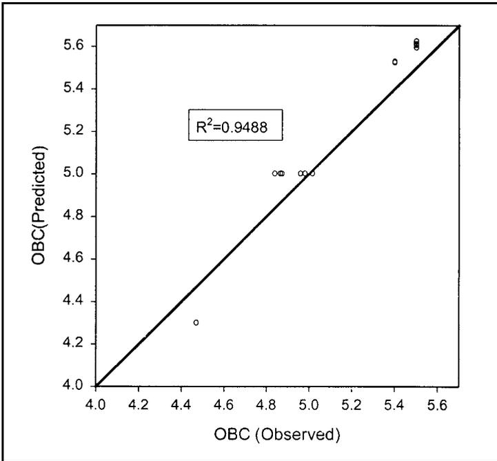
Fig. 7. The Correlation of Predicted to Observed OBC for Asphalt-Concrete Type IV.
