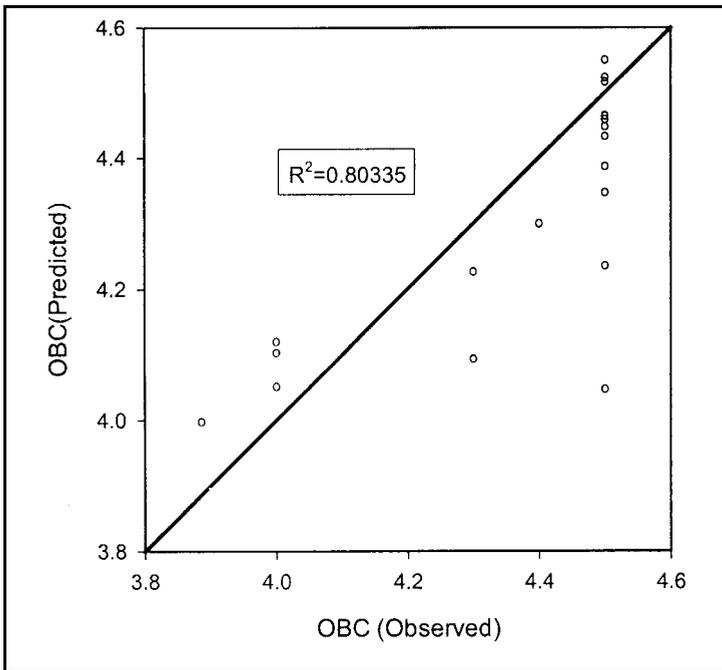
Fig. 5. The Correlation of Predicted to Observed OBC for Asphalt-Concrete Type II.
