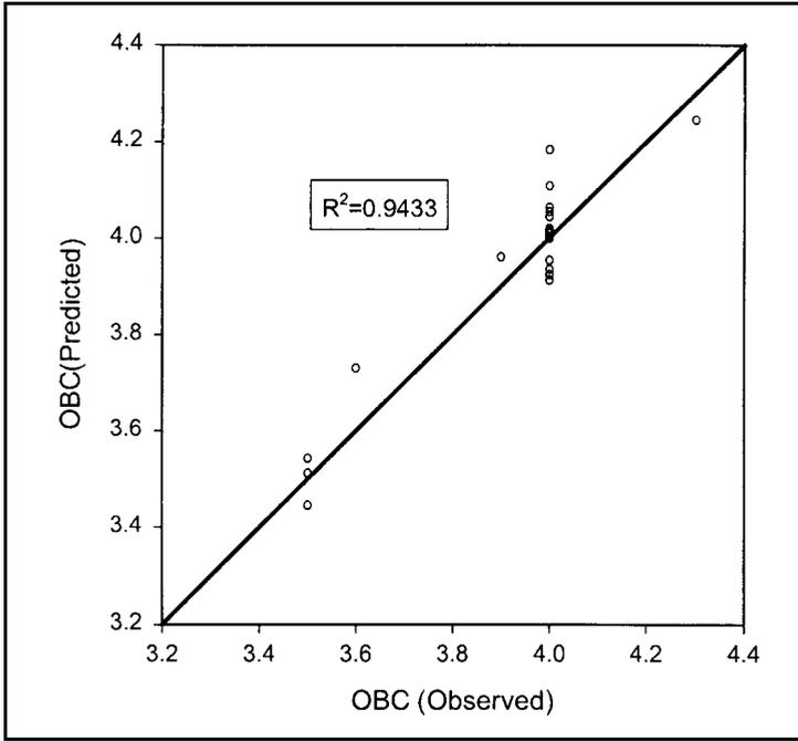
Fig. 4. The Correlation of Predicted to Observed OBC for Asphalt-Concrete Type I.
