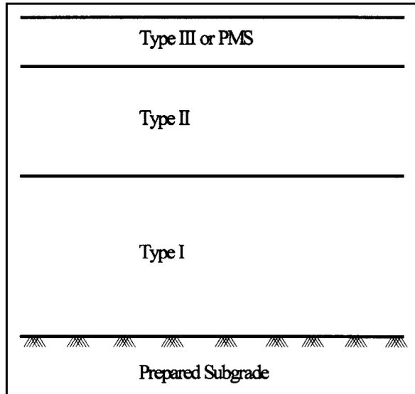
Fig. 2. A Typical Pavement Section in Kuwait.
