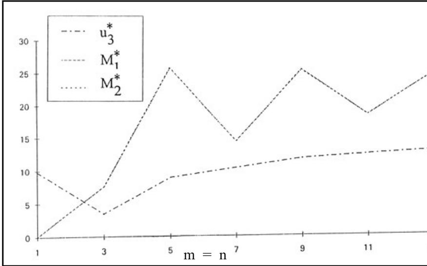
Fig. 5. Convergence of  $u_3^*$ ,  $M_1^*$  and  $M_2^*$  with  $m = n$ ,  $\frac{l_2}{l_1} = 1$ ,  $l_1/l_3 = 50$  and  $r/l_1 = 1000$ .
