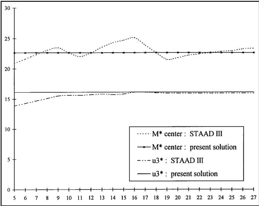
**Fig. 17.** Comparison of present and STAAD-III solutions for  $u_3^*$ , and  $M_1^*$  (central values) of cylindrical panel with  $\frac{l_1}{l_3} = 20$ ,  $\frac{l_2}{l_1} = 1$ , and  $\frac{r}{l_1} = 10$ .
