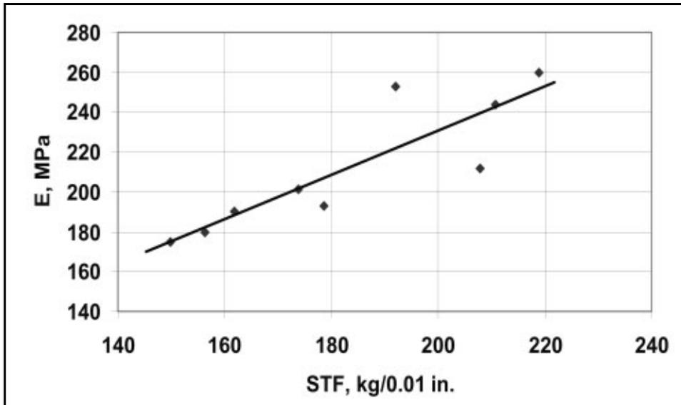
Fig.2. E versus STF at 60°C and 1.0 Hz
