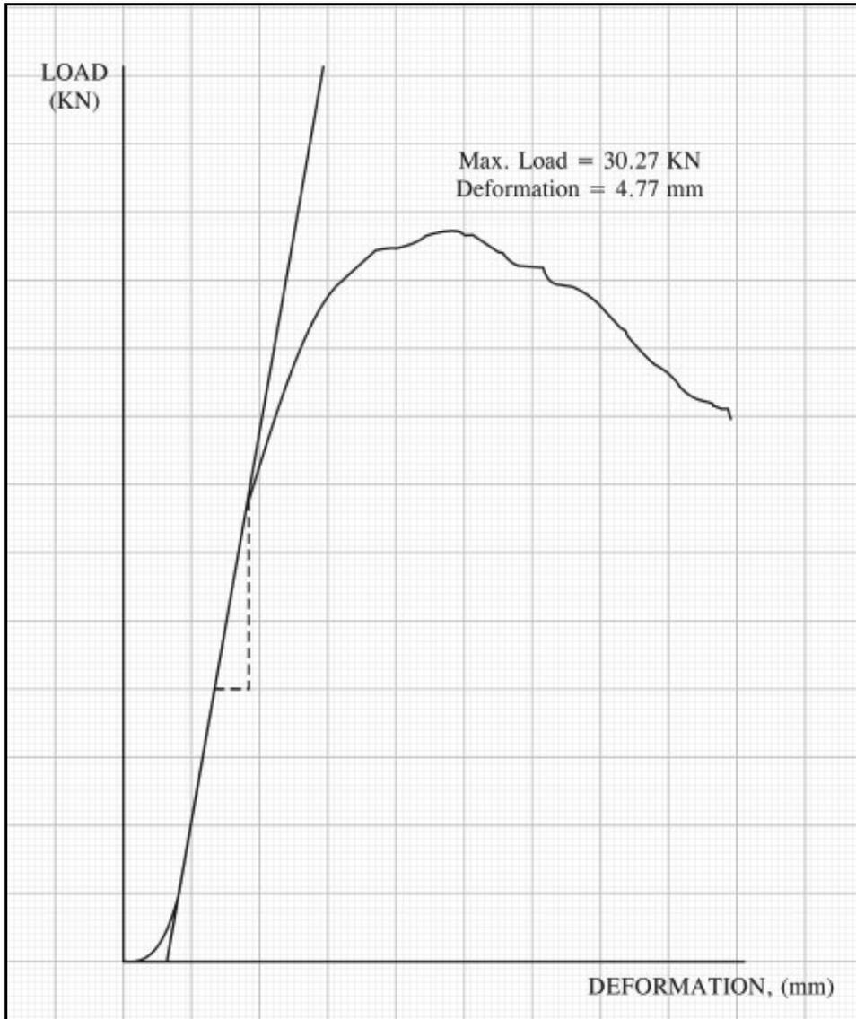
**Fig.1.** Marshall load-deformation curve for sample A1 of AC mix type I at 5.0% asphalt cement content
