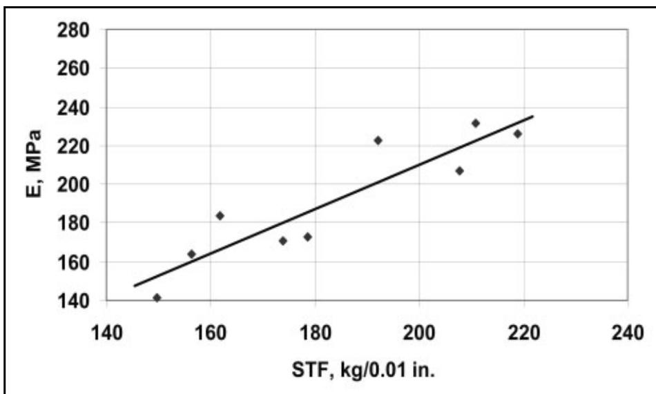
Fig.4. E versus STF @ 60°C and 0.33 Hz
