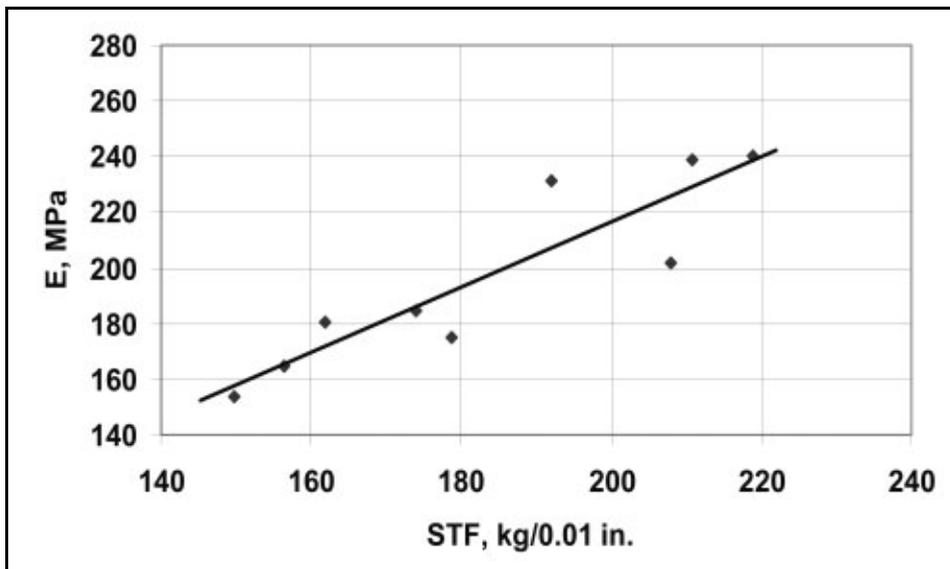
Fig.3. E versus STF at 60°C and 0.5 Hz
