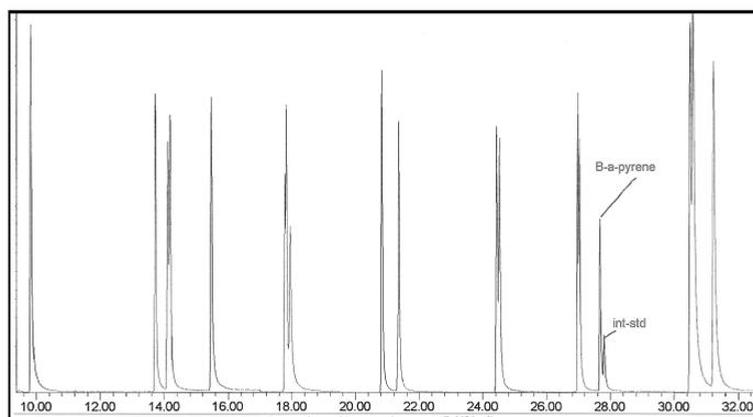
**Figure 1:** Chromatogram of standard PAHs along with all characteristic internal standard ions. GC/MS conditions: Column, DB-5 capillary column; GC oven temperature program, initial temperature 45<sup>0</sup>C; initial time, 2.00 min: Rate 10<sup>0</sup>C/min, final Temperature, 290<sup>0</sup>C; Final Hold Time, 8 min, Total Run Time, 33.70 min.
